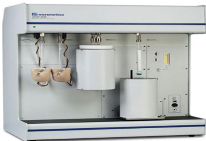
Fig. 6 Micromeritics ASAP 2020 Accelerated Surface area and porosimetry (Hernández 2016)
