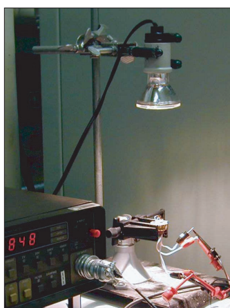
Figure 4 Voltage and power produced by a thermoelectric microdevice on illumination by a lamp.
