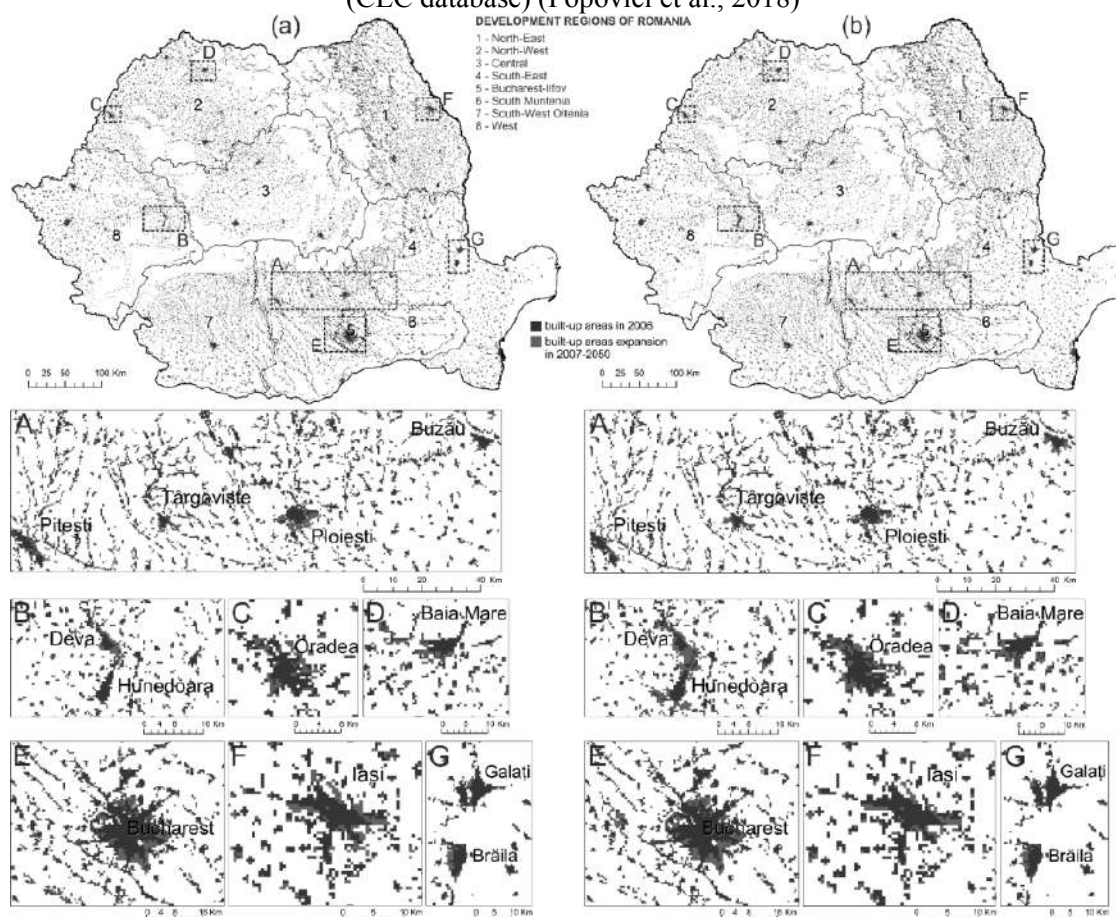
Figure 2. The built-up areas expansion (2007-2050) period based on CLUE-S model
