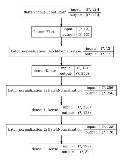
Fig. 8. Artificial neural network layer structure and data dimensions
