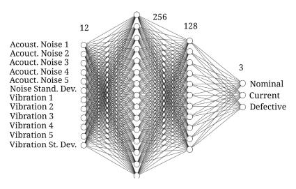
Fig. 7. Structure of neural connections
