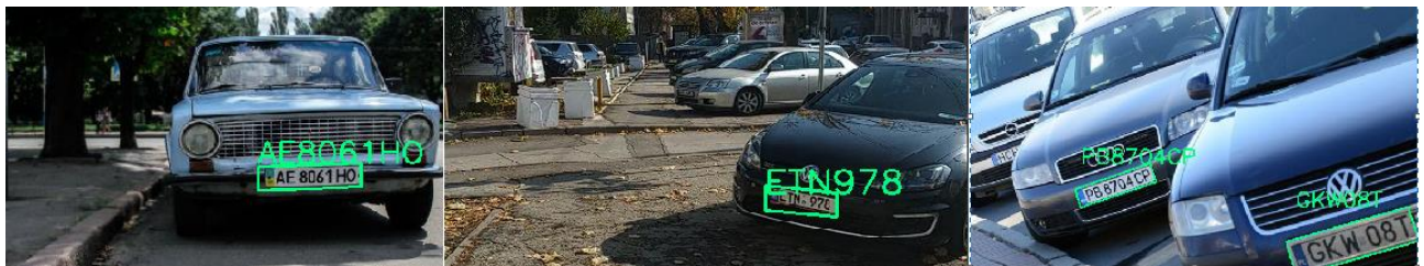
Figure 2. Examples of numberplate recognition from some photos
