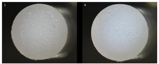
Fig. 5 Detail observed on the surface of the PE pins №1 and №4 following 2.5 Mc of testing (10X magnification).
