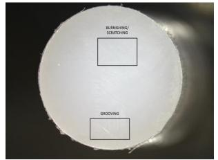
**Fig. 4** Damage observed on wear station PE pin following 28 days of testing (10X magnification).
