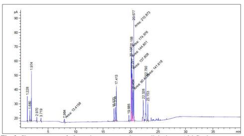
Fig. 3. Chromatogram of formed gases at petroleum radiolysis at 6.0 kGy dose.
