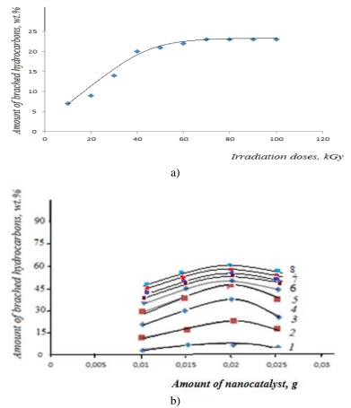
**Fig. 1.** a) - dependence of quantity of branched hydrocarbons and gamma quantum dose (irradiation without nanostructured sodium - bentonite clay); b) - dependence of quantity of branched hydrocarbons and the catalyst mass at doses: 1- 0.7 kGy; 2- 2.5kGy; 3- 4.5 kGy; 4- 6.0 kGy; 5- 20 kGy; 6- 40kGy; 7-70kGy; 8- 100kGy, m<sub>cat.</sub> = 0.01-0.025 g.
