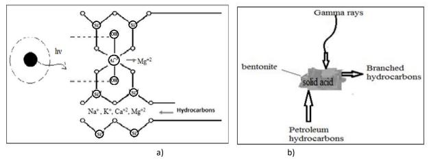
**Fig.2.** Transformation of hydrocarbons on the nanocatalyst (Na-bentonite): a) Hydrocarbons penetration in clay's pores; b) Formation of brunched hydrocarbons on the surface of solid acid – bentonite.
