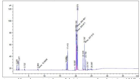
Fig. 4. Chromatogram of formed gases at petroleum radiolysis in presence of nanobentonite at 6.0 kGy dose.
