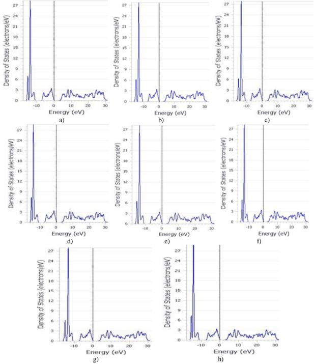
Fig. 4. Density of states calculation of LDA CAPZ functional with different Pseudopotentials for GaN for 5 ×5 ×4 k-points (a) OTFG Ultrasoft Schroedinger (b) OTFG Ultrasoft Koelling- Harmon (c) OTFG Ultrasoft Zora (d) OTFG norm conserving Schroedinger (e) OTFG norm conserving Koelling- Harmon (f) OTFG norm conserving Zora (g) ultrasoft Schroedinger / Koelling- Harmon/ Zora (h) norm conserving Schroedinger / Koelling- Harmon / Zora.
