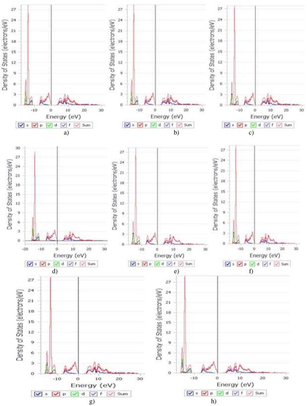
Fig. 5. Partial Energy Density of states calculation of LDA CAPZ functional with different Pseudopotentials for GaN for 5 ×5 ×4 k-points (a) OTFG Ultrasoft Schroedinger (b) OTFG Ultrasoft Koelling- Harmon (c) OTFG Ultrasoft Zora (d) OTFG norm conserving Schroedinger (e) OTFG norm conserving Koelling- Harmon (f) OTFG norm conserving Zora (g) ultrasoft Schroedinger/Koelling- Harmon/Zora (h) norm conserving Schroedinger/Zoralling- Harmon / zora.
