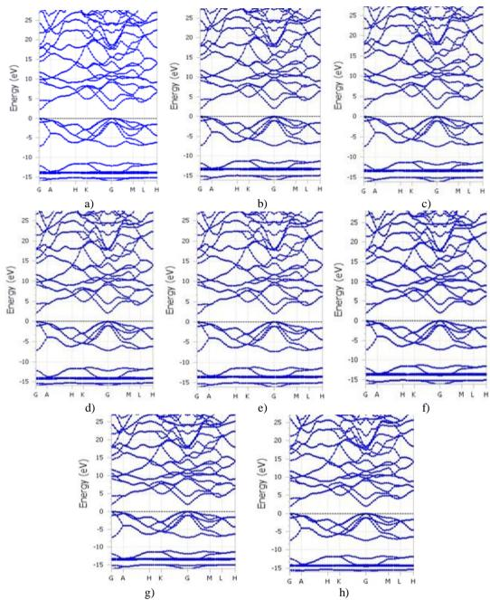
Fig. 3. Band gap calculation of LDA CAPZ functional with different Pseudopotentials for GaN for 5 ×5 ×4 k-points (a) OTFG Ultrasoft Schroedinger (b) OTFG Ultrasoft Koelling- Harmon (c) OTFG Ultrasoft Zora (d) OTFG norm conserving Schroedinger (e) OTFG norm conserving Koelling- Harmon (f) OTFG norm conserving Zora (g) ultrasoft Schroedinger / Koelling- Harmon/ Zora (h) norm conserving Schroedinger / Koelling- Harmon / Zora (Table – 1).
