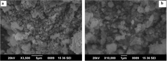
Fig. 6. Scanning electron microscopy images of synthesized silver nanoparticles.
