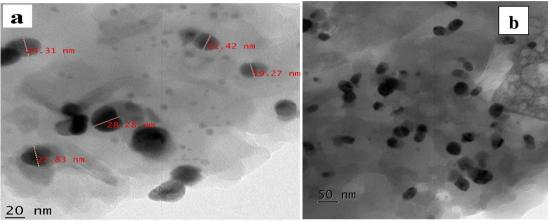
Fig. 4. TEM Images of synthesized silver nanoparticles at 20 and 50 nm scale.
