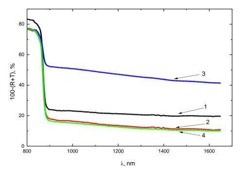
**Fig. 5.** Absorption spectra of single crystals *p*-CdTe (111): original sample is curve 1 and the samples are irradiated with energy of 66 mJ/cm<sup>2</sup>; 108 mJ/cm<sup>2</sup>, 164 mJ/cm<sup>2</sup> - curves 2-4 respectively.
