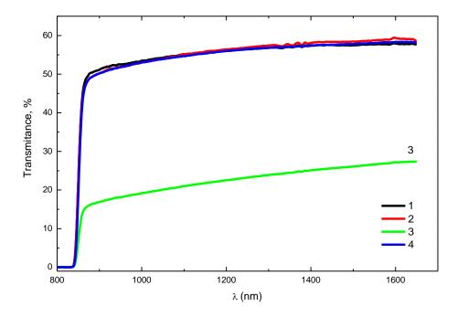
**Fig. 1.** Transmission spectra of single crystals *p*-CdTe (111): original sample is curve 1 and the samples are irradiated with energy of 66 mJ/cm<sup>2</sup>; 108 mJ/cm<sup>2</sup>, 164 mJ/cm<sup>2</sup> - curves 2-4 respectively.
