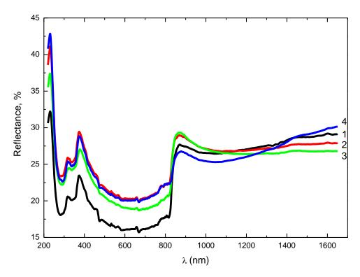
Fig. 4. Reflection spectra of solid solutions  $Cd_{1-x}Zn_xTe$  (x = 0.1): original sample is curve 1 and the samples are irradiated with energy of 46.66 mJ/cm<sup>2</sup>; 102.3 mJ/cm<sup>2</sup>, 163.5 mJ/cm<sup>2</sup> - curves 2-4 respectively.
