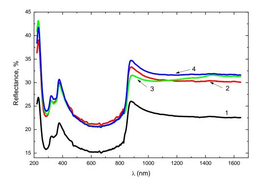
**Fig. 3.** Reflection spectra of single crystals *p*-CdTe (111): original sample is curve 1 and the samples are irradiated with energy of 66 mJ/cm<sup>2</sup>; 108 mJ/cm<sup>2</sup>, 164 mJ/cm<sup>2</sup> - curves 2-4 respectively.
