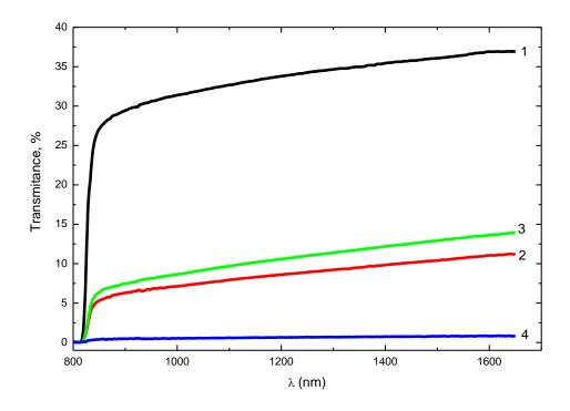
Fig. 2. Transmission spectra of solid solutions  $Cd_{1-x}Zn_xTe$  (x = 0.1): original sample is curve 1 and the samples are irradiated with energy of 46.66 mJ/cm<sup>2</sup>; 102.3 mJ/cm<sup>2</sup>, 163.5 mJ/cm<sup>2</sup> - curves 2-4 respectively.
