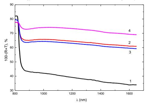
Fig. 6. Absorption spectra of solid solutions  $Cd_{1-x}Zn_xTe$  (x = 0.1): original sample is curve 1 and the samples are irradiated with energy of 46.66 mJ/cm<sup>2</sup>; 102.3 mJ/cm<sup>2</sup>, 163.5 mJ/cm<sup>2</sup> - curves 2-4 respectively.
