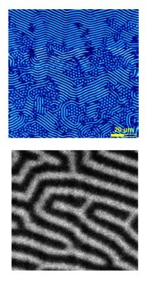
**Fig. 2.** Image of the labyrinth domain structure of the YIG films.
